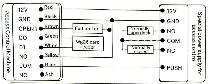
The signal output by the door access control machine is a relay signal, which can directly drive electric locks, automatic doors, barrier gates and other equipment. Please consult the supplier for the specific wiring method.
